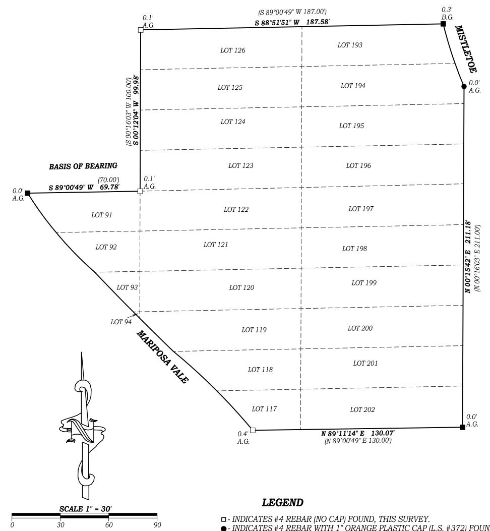
•- INDICATES #4 REBAR WITH 1" ORANGE PLASTIC CAP (L.S. #372) FOUND, THIS SURVEY.
